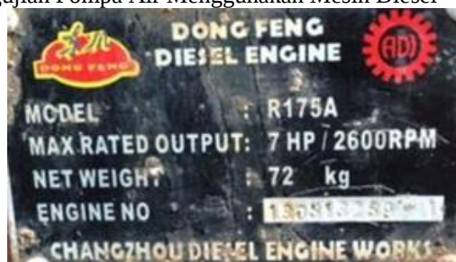
Gambar 3: Name Plate Mesin Diesel
