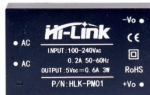
Gambar 4. HLK-PM01 AC-DC (Sumber : Datasheet HLK-PM01 AC-DC)
