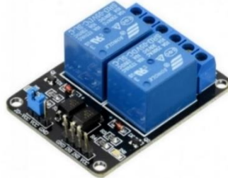
Gambar 3. Relay 2 Channel (Sumber : Datasheet Relay 2 Channel)
